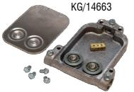
Cable tee pulley (KG/14663) will accept a KG/14682 T-handle cable pull rope as input and two KG/14668 extender cables as outputs. This permits one T-handle to pull the cotter pins of two manual head activators.
