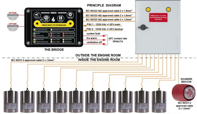
This schedule of working principles of the NANO fire extinguishing system is intended to be supportive of this leaflet and therefore not intended and suitable for technical realization. For more detailed information ask for the User Manual NANO-EN August 2022 V1.0 and contact the K&G Groep BV.
