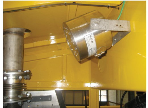
Photo of the engine compartment. The generator is mounted to the upper right. The control panel used is SP-1 and detection is made with heat sensitive cable
