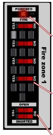
These resistors are also present on the  $\mu$ -FTM test module. All possible alarms and faults can be simulated by using the switches.
