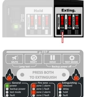
In the event of a fire alarm in both fire alarm zones or when the **'PRESSED' 'EXTING'** switch is in the **YES** position, and an extinguishing release delay is programmed, then the red 'delay' LED is lit in the 'Extinguishing' group. When operating the **'PRESSED' 'HOLD'** switch, the tone signal will change, and the yellow 'hold' LED is lit in the 'Extinguishing' group. This operation does not apply when DIP switches 7 & 8 are programmed. Refer to the µ-FEP manual for this.
