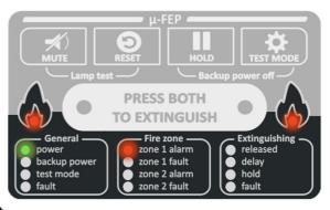
A cable malfunction can be simulated by setting the red **'SHORTED'** switch to the **YES** position. A fault indication in 'fire zone 1' is the result. There are two yellow LEDs lit, one (fault) in the 'General' group and the other (zone 1 fault) in the 'Fire zone' group.
