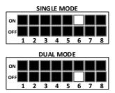
In dual (standard) mode the extinguisher(s) will be released after both detection zones will have a fire alarm condition and cause an internal pulsing alarm sound. The fire relay and extinguisher are activated according to the dip-switch settings. In single mode the extinguisher(s) will be released when one detection zone is in fire alarm condition and cause an internal pulsing alarm sound. The fire relay and extinguisher are activated according to the dip-switch settings.
