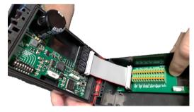
Mount the rear part (backbox) at the desired location. The hinged catch of this enclosures conceals the installation screws. Connect the required cables with sufficient length and connect them to the terminal block according to the connection requirements. After the cable glands have been tightened, the front part with the electronics must be reinstalled and the flat cable must be re-connected.
