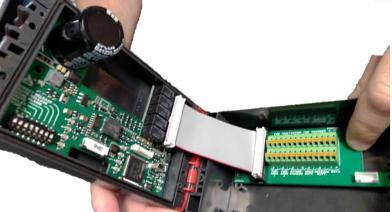
After the cable glands have been tightened, the front part with the electronics must be re-installed and the flat cable must be re-connected.
