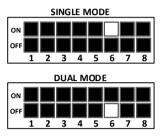
In dual (standard) mode the extinguisher(s) will be released after both detection zones will have a fire alarm condition and cause an internal pulsing alarm sound. The fire relay and extinguisher are activated according to the dip-switch settings. In single mode the extinguisher(s) will be released when one detection zone is in fire alarm condition and cause an internal pulsing alarm sound. The fire relay and extinguisher are activated according to the dip-switch settings.
