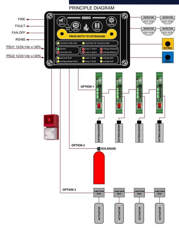
This diagram of the working principles of the NANO fire detection & extinguishing system is intended to support this leaflet and is therefore not intended or suitable for technical implementation. For more detailed information, please request the NANO User Manual.
