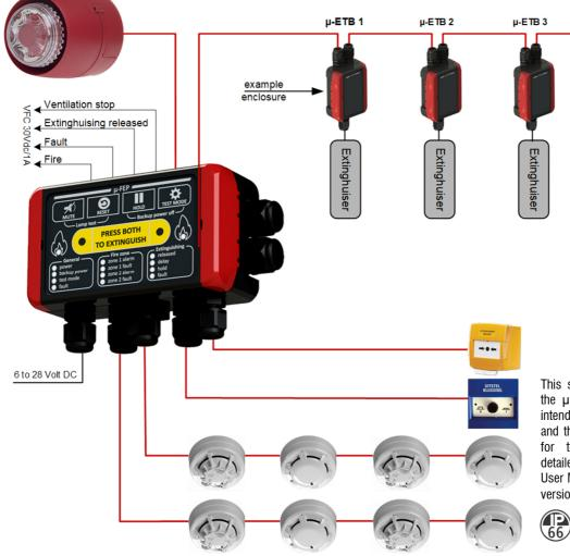
This schedule of working principles of the  $\mu$ -FEP fire extinguishing system is intended to be supportive of this leaflet and therefore not intended and suitable for technical realization. For more detailed information ask for the K&G User Manual  $\mu$ -FEP-EN, March 1, 2021 version 1.10
